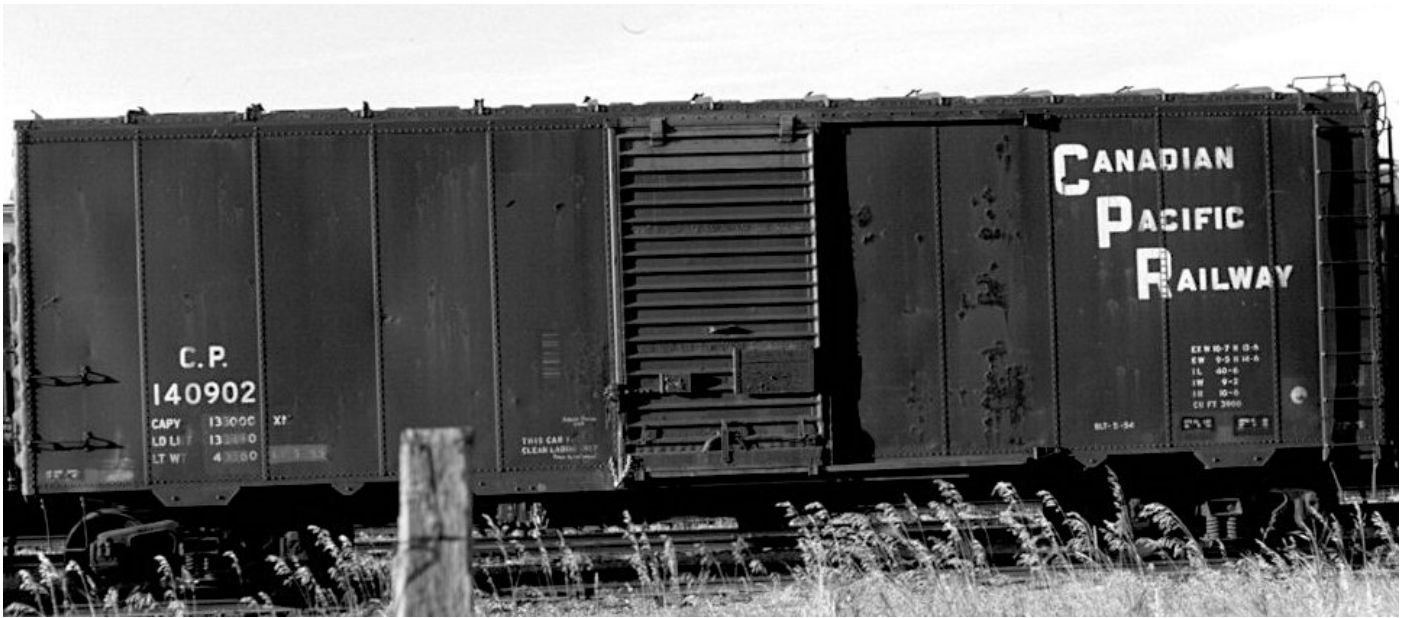
CP 140902 WITH 4-4 IDE ENDS IS SHOWN TO ILLUSTRATE THE 3 STEP BLOCK LETTERING SCHEME, BOWNESS, AB. AUGUST 9, 1991. ANDY J. BROSCOE PHOTO.
