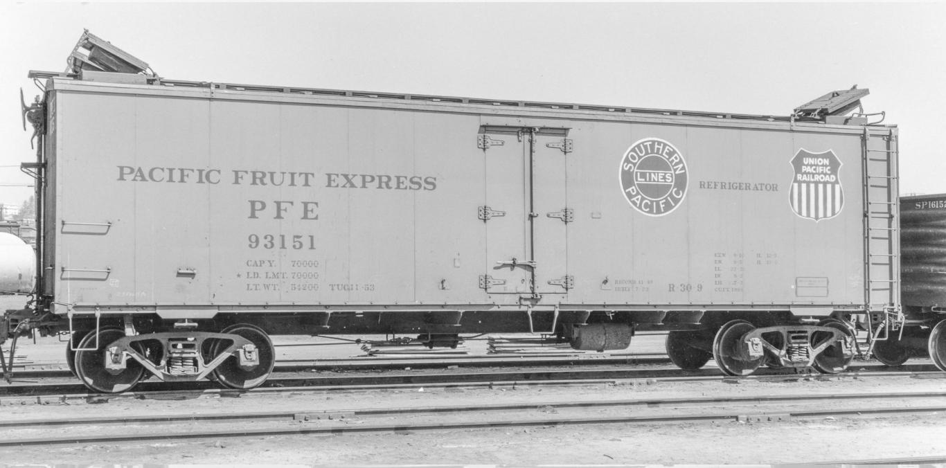
At the same time that the -24s were being rebuilt, many refurbished -9 cars required service. Numerous -9s received plywood side sheathing in the late 1940s. The ends retained tongue and groove sheathing boards. Documented car nos. include 93151 shown above, as well as 91593, 94242, 94789 (page 247, *PFE, 2nd Ed.*,) and 64771 (a -21 rebuild.) For more info, see page 148 of *PFE, 2nd Ed*.
