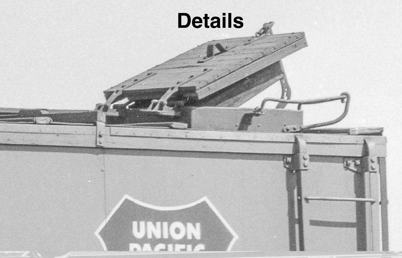
Again, note the ladder brackets, roof grab iron, and the hatch cover rest
